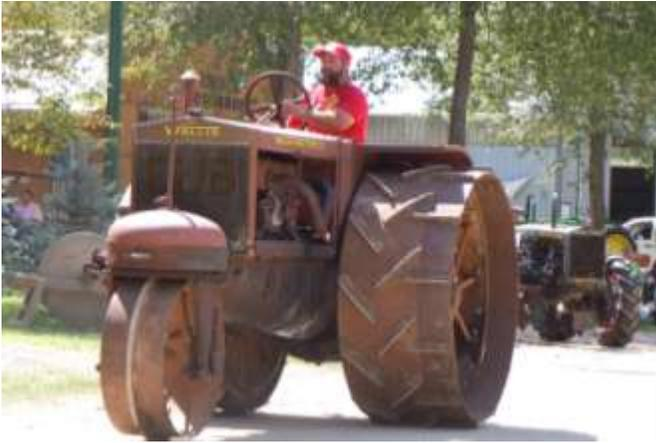
Joe Poncelet of Lake City, MN exhibited his 48 hp 1917 Wallis Cub, complete with the little cub in front, which indicates the direction of the front wheel for steering.
