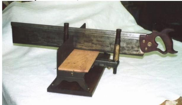
*Donated by an unknown person, this cast iron miter box was manufactured by Langdon Miter Box Co. of Miller Falls, Mass., pat'd 1896. Langdon was the first to build an all metal miter box.*
