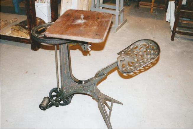
This Barnes Foot Powered Mortising Machine was donated to the Club by Jim Allen of Necedah. It was built in Rockford, Illinois and carries a patent date of 1879. This machine runs fine and does a nice job on making molding used by cabinet makers.
