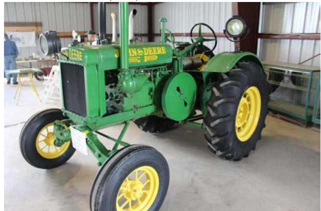
Interesting, but a little scary, this 1933 GP tractor has an acetylene lighting system, which includes lights on the front, fender and tail. It is owned by Randy Eggimann of Cape Girardeau, MO.
