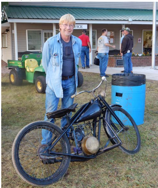
From way up north, exhibitor Bob Gale shows off his unusual 1938 Simplex Servi-Cycle. It weighs only 148 lbs. and has a 125cc engine.
