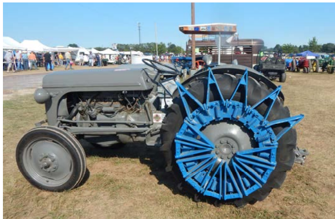
This very interesting Ferguson attachment could convert a rubber tire to a spaded wheel, using hinged spades. It is mounted on a Ferguson TO20 tractor owned by William Rupnow.
