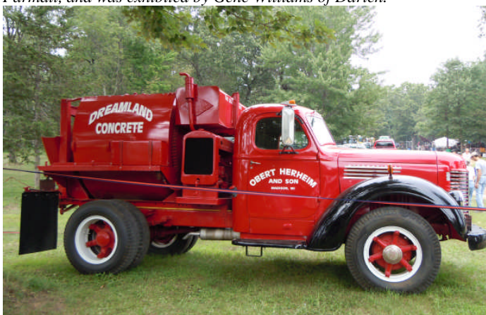
I never thought I would fall in love with a concrete truck, but this one stole my heart... it's a 1947 IH truck, with a Blaw-Knox 1.5 cubic yard mixer powered by a 1940 12 hp Hercules engine. The owner is Obert Herheim of Madison. And it's such a beautiful shade of red too...
