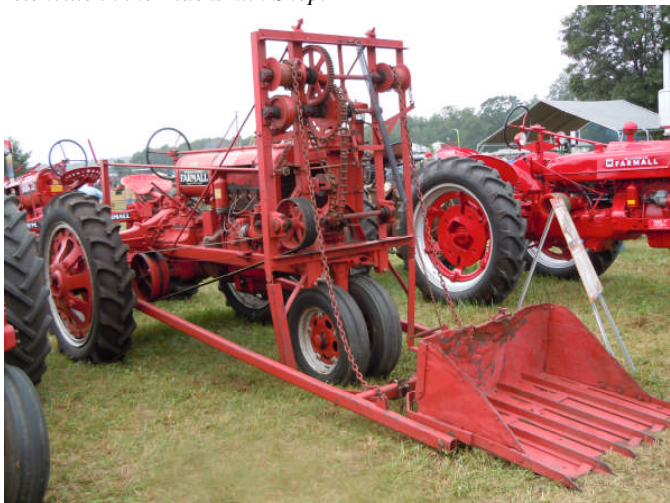
Interesting comments can be heard while standing by this exhibit! The Farmer's Friend Tractor Power Fork & Shovel was made by G&D Manufacturing Co. of Streator, IL. It is installed on a 1938 F-20 Farmall, and was exhibited by Gene Williams of Darien.
