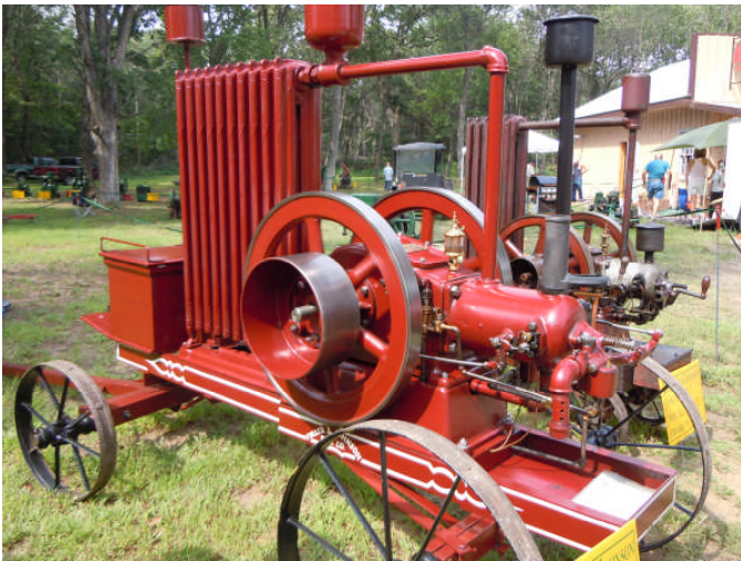
Don Winkler displayed this 1904 3 hp Fuller & Johnson oil cooled gas engine.
