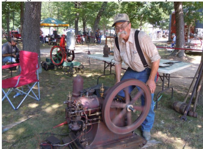
Jim Keats displayed his 1905 2 hp National Engineering engine, made in Saginaw, MI. It has a pendulum governor, rare on a small engine.
