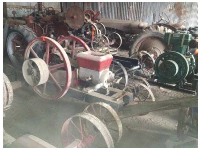
6 hp Associated engine, with rebuilt igniter and on a cart.
