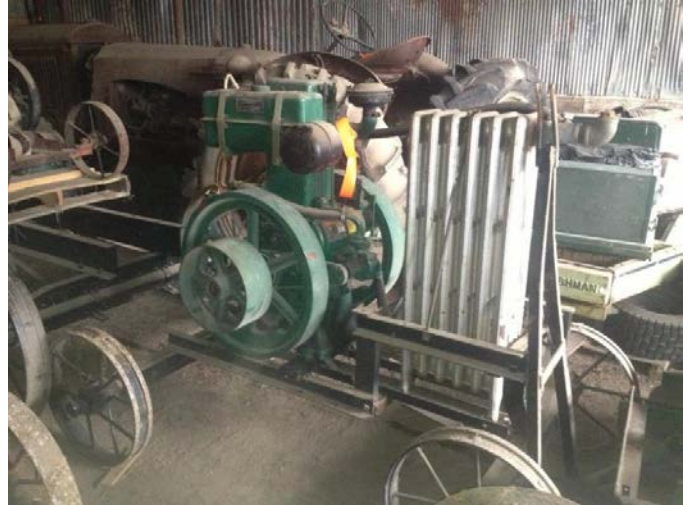
6 hp Fieldmarshal diesel with cart and radiator. This is a newer engine from India.
