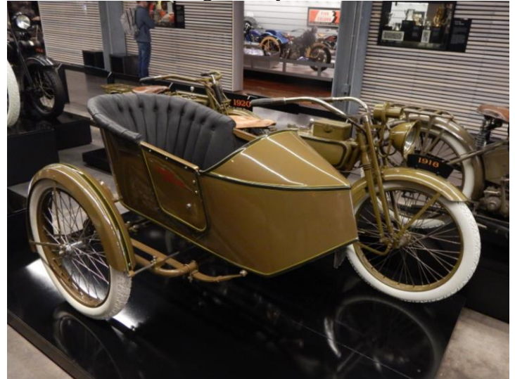
This 1918 Model J sports a beautifully upholstered J.W. Rogers side car, a $90 extra. A special engine with more torque was recommended to accommodate the side car.
