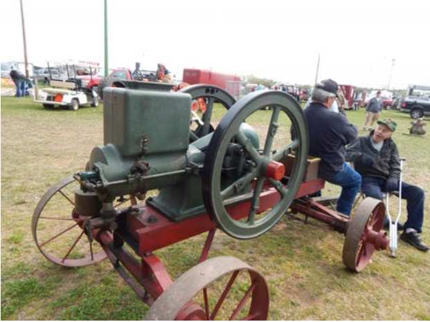
Waiting for the auction to begin is easier when you have a rare gas engine to perch on. This is a 7 hp Steiner "Longlife" engine, made by Steiner Mfg. Co. of Plymouth, WI.
