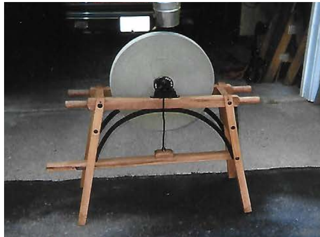
This foot-powered emery stone was donated to the Club by Peter Holzman. The patent date is May 4, 1884 and the stone has the date 1887 carved in it. The wood was all replaced by Club members Lyle Opperman and Don Blausey. Photo courtesy of Lyle Opperman
