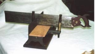
Donated by an unknown person, this cast iron miter box was manufactured by Langdon Miter Box Co. of Miller Falls, Mass., pat'd 1896. Langdon was the first to build an all metal miter box. Courtesy of Lyle Opperman
