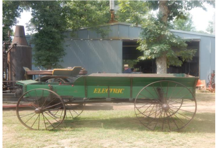
This "Electric" wagon is in amazing original condition. It was manufactured by the Electric Wheel Co. of Quincy, IL which was founded in 1890. The company was an early manufacturer of steel wheels and "Electric" probably referred to the electric welding process which was new at the time. Richard Thomas of Roselle, IL is the owner of this extraordinary early piece.
