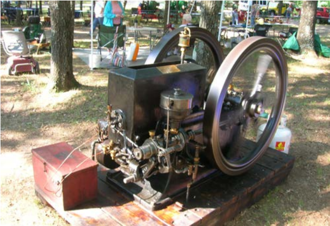
This rare 6 hp Fairbanks cam stopper engine (not connected to Fairbanks Morse) was manufactured in New York. It was displayed by Bill Winkler.
