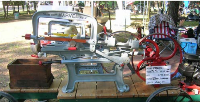
James Wheeler of Dane brought this marvelous Marvel Draw Cut Saw, No. 2. It was patented in 1912.
