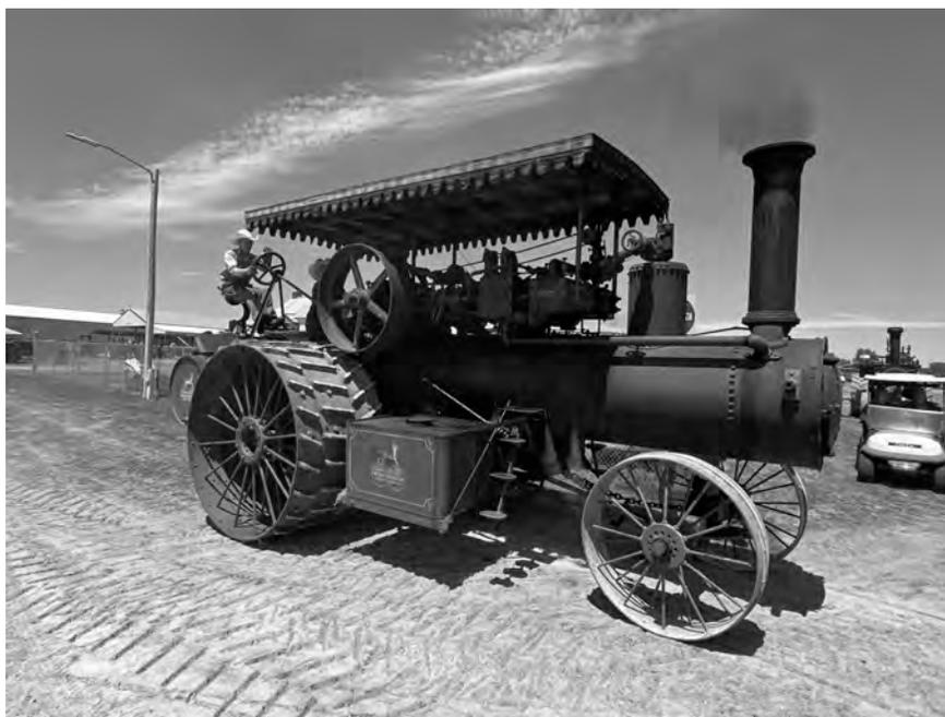
One of the many rarities that you will see at this year's show is this 40 horsepower Gaar-Scott steam traction engine. This engine was built in 1908 and was the largest of the Gaar-Scott line. It's one of two left in existence and the only one running. Owned and restored by Jerred Ruble of Hanlontown, IA. It and Jerred's 36 horsepower Rumely steam engine will be the largest engine at this year's show.
